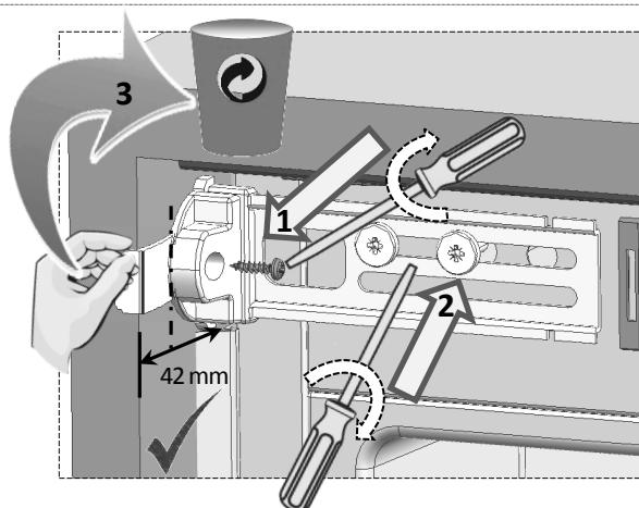
*Installation step for 16: screws should be fully tightened at this stage.*
