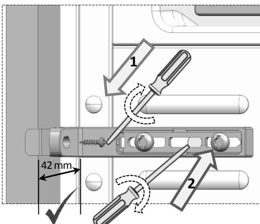
*Installation step for 14: screws should be fully tightened at this stage.*
