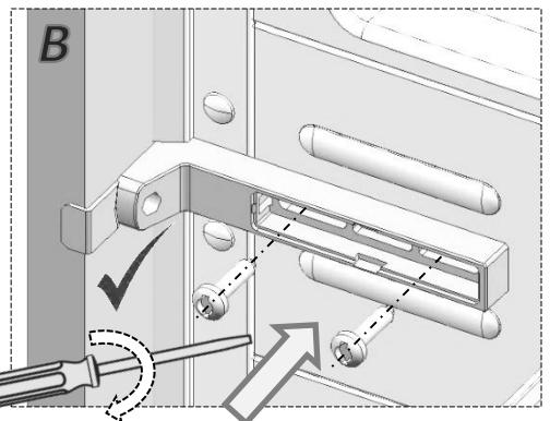
*Installation step for 13\_B: screws should not be fully tightened at this stage.*
