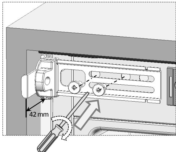
*Installation step for 15: screws should not be fully tightened at this stage.*
