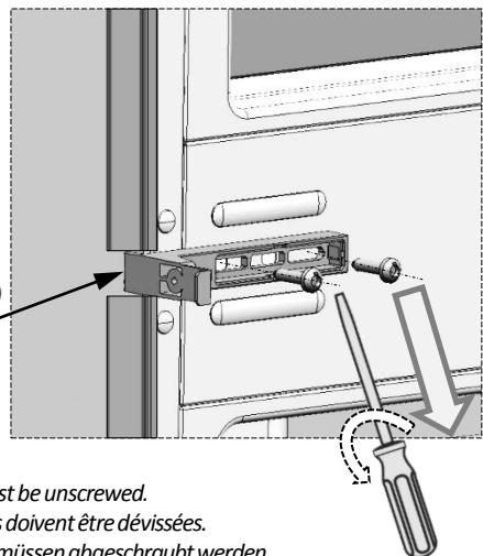
**Installation step for 10:** screws must be unscrewed.
