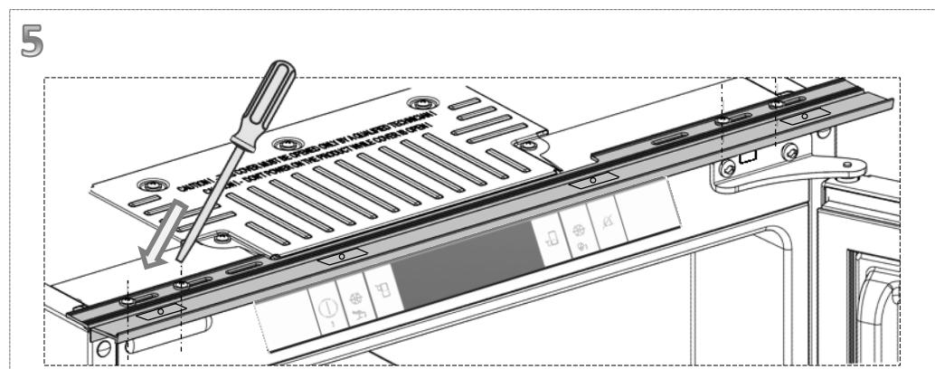
**Note:** screws for connecting top plastic part should not be screwed very hard, because of moving the plastic part easily left or right side.
