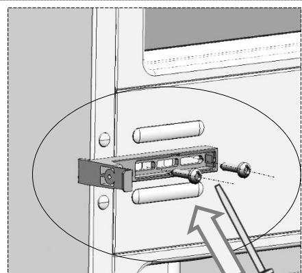
*Installation step for 7: screws should not be fully tightened at this stage.*
