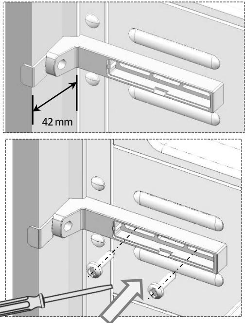
*Installation step for 13: screws should not be fully tightened at this stage.*
